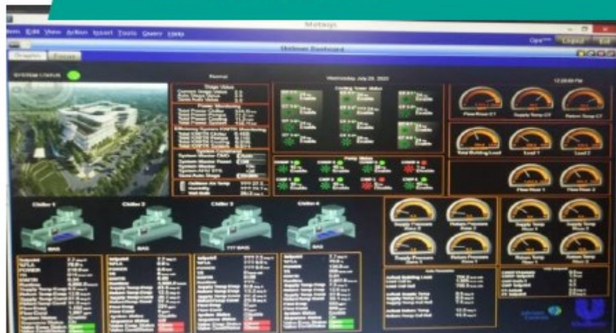
Figure 4-4. Chiller Optimizing Plant GU Office Building
