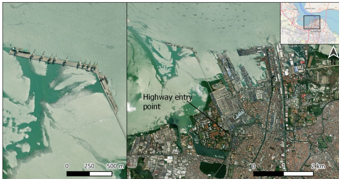
Figure 16. A satellite image of the Port of Surabaya. Entry/exit road at the western part of the port and entry of the highway are in line, which makes this port suitable for transportation of long wind turbine components.
