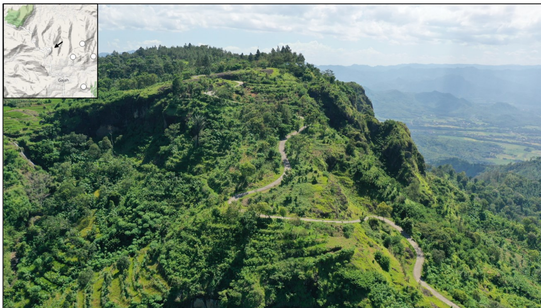
Figure 10. Existing road from Bungkal, which connects the plains around Ponorogo to the plateau (650-800 height difference). The cliffs on the left and the right side of the road are not represented in height models. Inclination of the road is estimated to be over 20% in some sections.
