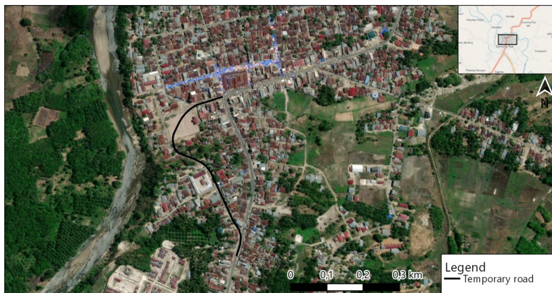
Figure 21. The black line represents a diversion from the main road; this uses mainly existing roads (~350 m), and 200 m of new temporary road over a square/parking lot.
