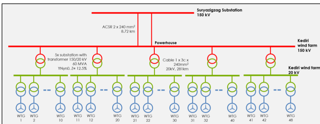
Figure 33. A schematic design of the transmission and distribution network at the envisioned Kediri wind farm
