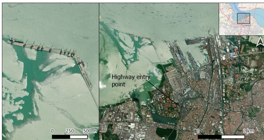
Figure 15. A satellite image of the Port of Surabaya. Entry/exit road at the western part of the port and entry of the highway are in line, which makes this port suitable for transportation of long wind turbine components.
