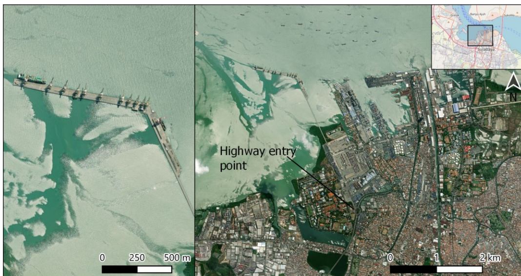
Figure 15. Port of Surabaya. Entry/exit road of western part of the port and entry of the highway are in line, which makes this port suitable for transportation of long wind turbine components.
