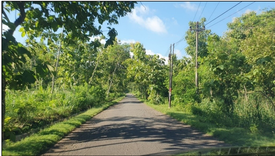
Figure 24. The road connecting Semanu to the villages within the site. Roads will have to be cleared of overhanging trees/branches and in the curves some widening might be necessary. It is expected that after construction, the whole road needs asphaltting due to the heavy transport.
