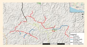
Within the site, new roads need to be constructed on hilly and steep areas, and some existing roads and bridges must be strengthened.
