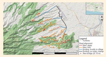
Within the site, new roads need to be constructed, and some existing roads and bridges must be strengthened.
