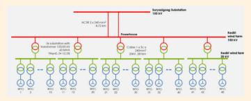
The closest point of connection to the existing grid is the Surya Zig Zag 150 kV PLN substation. From this PLN substation to the wind farm's powerhouse, a 9 km transmission line is required. The generated electricity will be distributed to the powerhouse via five wind farm substations.
