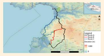
The Fishing Port of Pelabuhan Ratu is deemed to be the most suitable entry point of the turbines, with access to the site available via regional roads. Some challenges expected from the port exit to the site include a section of steep hills and cage design bridges.
