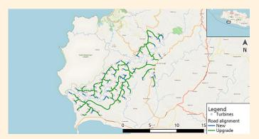
Within the site, new roads need to be constructed, and some existing roads and bridges must be upgraded in the rural parts.
