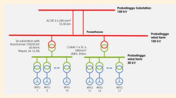
The closest point of connection to the existing grid is the Probolinggo 150 kV PLN substation. From this PLN substation to the wind farm's powerhouse, a 13 km transmission line is required. The generated electricity will be distributed to the powerhouse via two wind farm substations.
