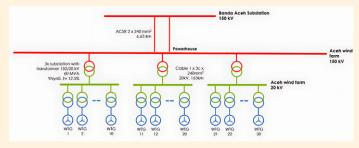
The closest point of connection to the existing grid is the Banda Aceh 150 kV PLN substation. From this PLN substation to the wind farm's powerhouse, a 6 km transmission line is required. The generated electricity will be distributed to the powerhouse via three wind farm substations.
