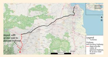
The Port of Surabaya is deemed to be the most suitable entry point of the turbines, with access to the site available via highway/toll road. No challenges expected from port until 25 km north of the site. A planned toll road until Kediri is in preparatory phase.
