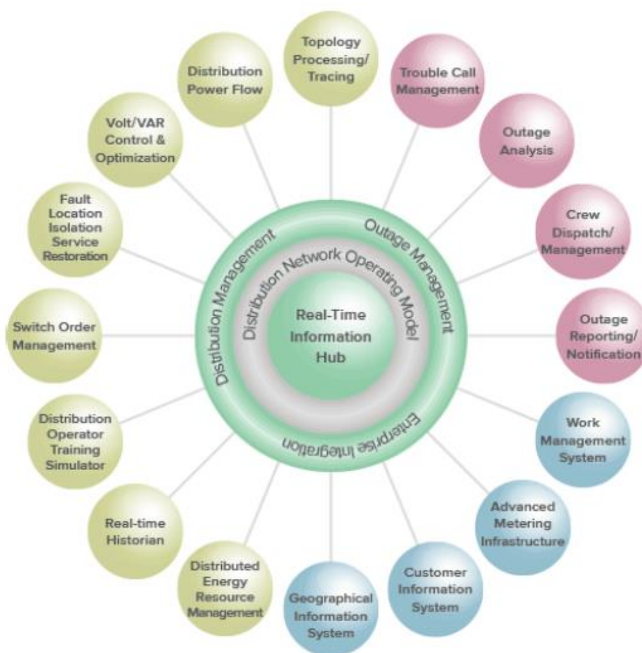
Figure 2-10 ILLUSTRATIVE ADMS INTEGRATION OF DISPARATE SYSTEMS, FUNCTIONS, AND
