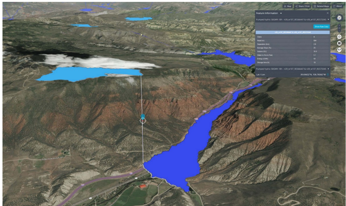
Figure 13. Individual greenfield site [16] showing upper reservoir (light blue), lower reservoir (dark blue), connecting tunnel route and information pop-up. Image credit: Data61 hosting and Bing Map background.
