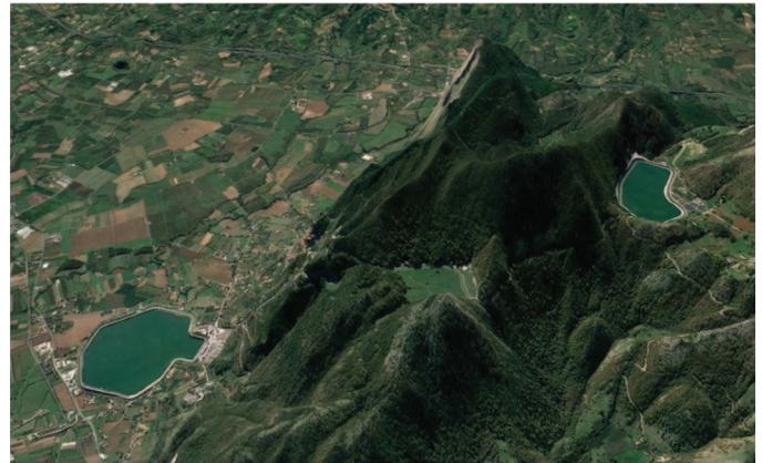
Fig. 2. Presenzano hydroelectric plant in Italy showing the reservoirs (upper right and lower left). This closed-loop pumped storage system has a head of 500 m, a power capacity of 1 GW, and storage of about 6 GWh (Google Earth image).
