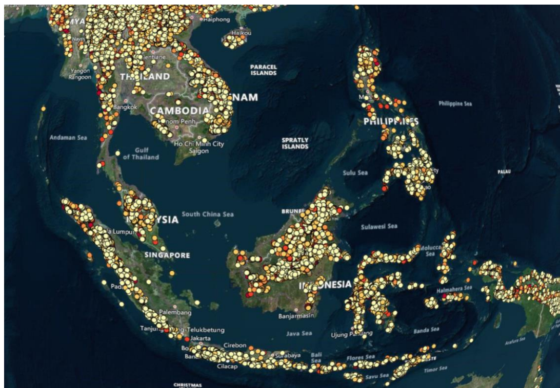
Figure 2 | 60,000 good sites for off-river Pumped Hydro Energy Storage, equivalent to 2 million Gigawatt-hours, in ASEAN according to an ANU's model.
