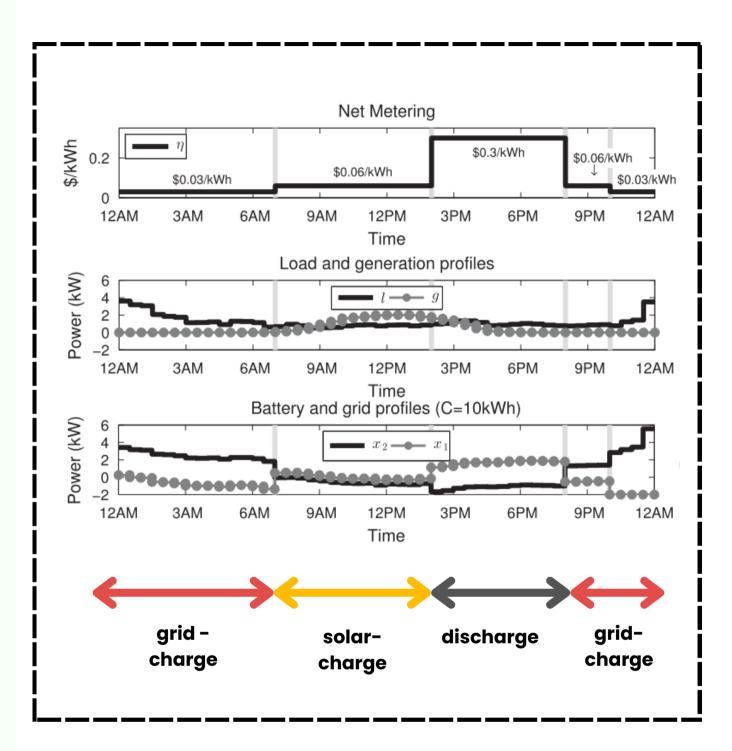
Financial policy, load and generation profiles, and grid and battery profiles for a battery of 10 kWh.
