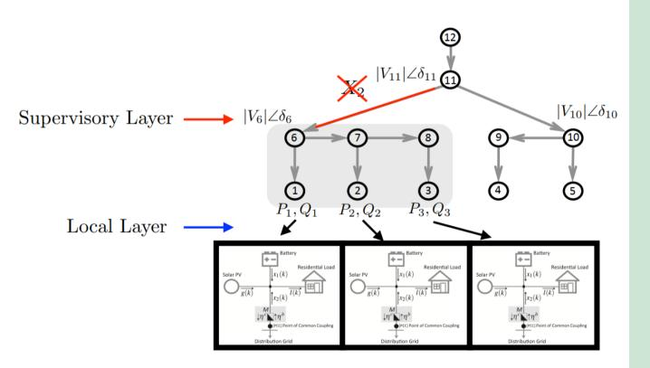
Source: Phasor-Based Control for Scalable Integration of Variable Energy Resources, A von Meier, EL Ratnam, K Brady, K Moffat, J Swartz, Energies 13 (1), 190 Synchronized phasors (synchrophasors) provide a real-time measurement of electrical quantities from across the power system.
